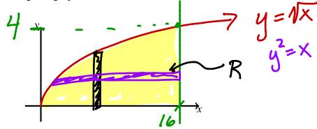
(b) **Use disks/washers** to completely set up, but not evaluate, a definite integral for the volume of the solid of revolution formed by rotating the region in part (a) around **the x-axis**.
